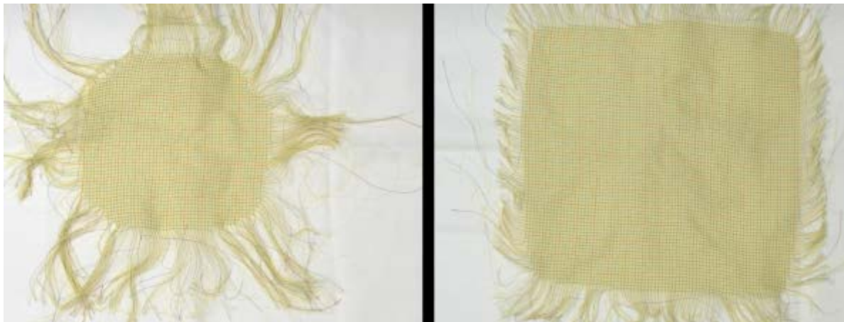
"Gentler" comparison based on AHAM mechanical action analysis. 1) Speed Queen TR5 score = 45.25; 2) Competitor Z score = 79.17
